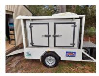
The trailer was professionally wired to run on 240 volts, either from a 15 amp mains source or it can be connected to a suitable portable generator which can be housed in a locked cabinet on the front drawbar.
